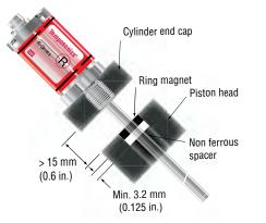
Figure 1. Model RH rod-style mounting
