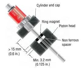
Figure 7. Model EH rod-style mounting
