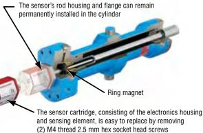
Figure 2. Fluid cylinder installation
