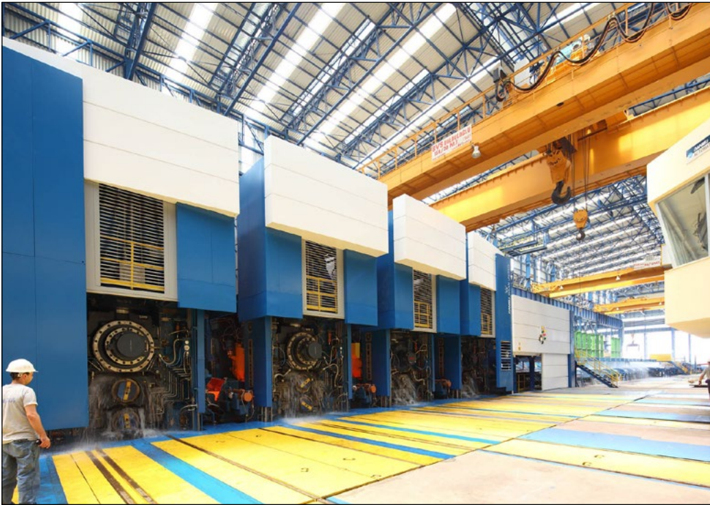
Fig. 1: Precise roll gap control with Temposonics position sensors
