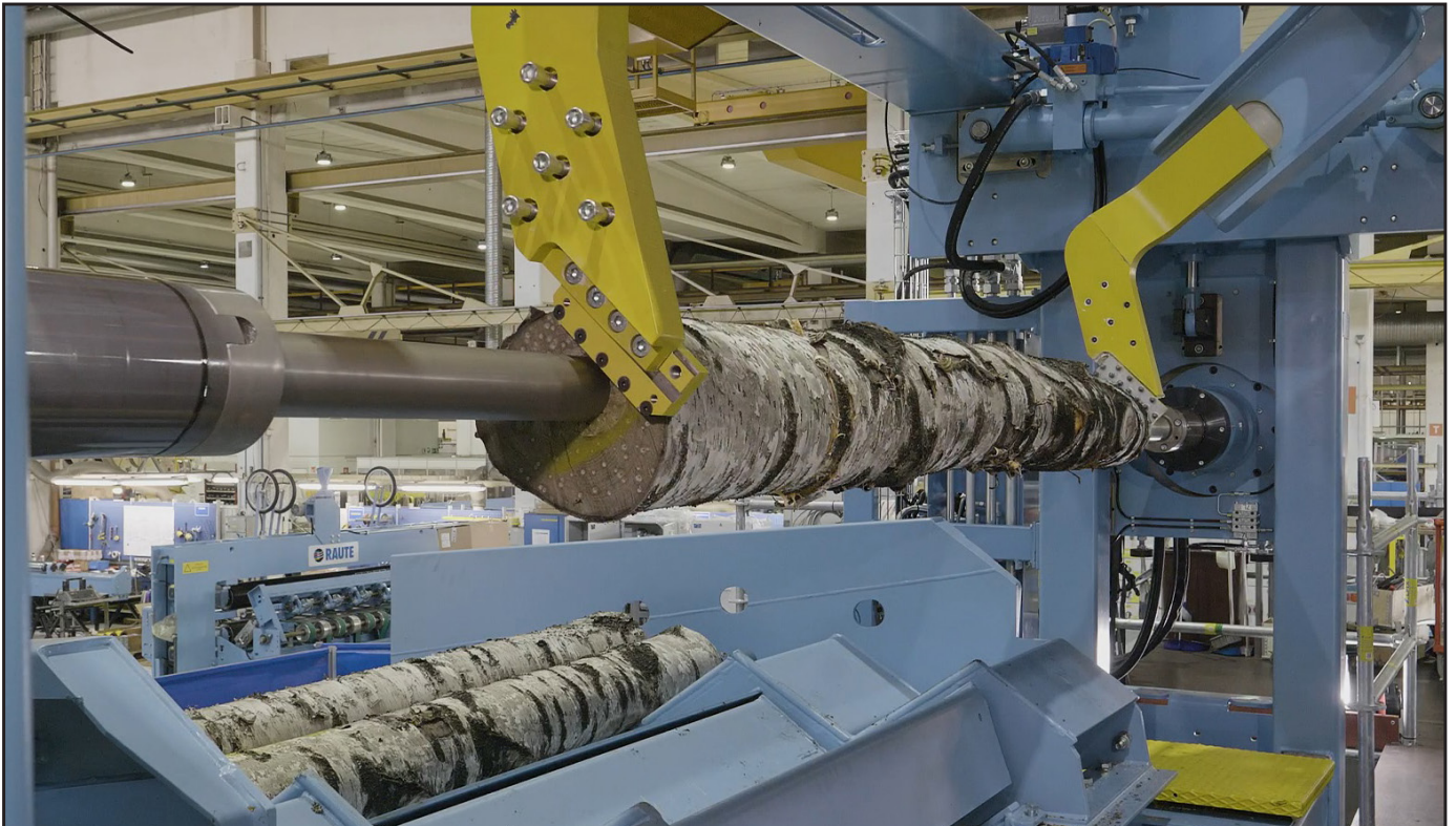
Fig. 1: Veneer peeling application
