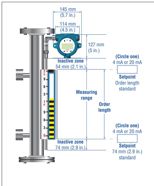
Fig. 1: Electronic mounting style "4" (top right)
