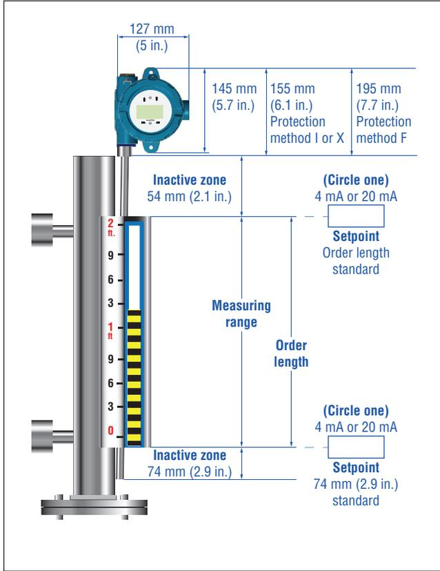
Fig. 3: Electronic mounting style "7" (top mount)
