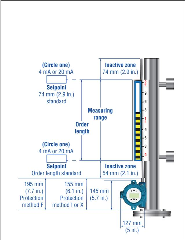
Fig. 4: Electronic mounting style "8" (bottom mount)
