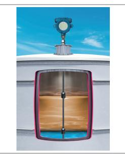
Fig. 3: Example of product and interface level measurement
