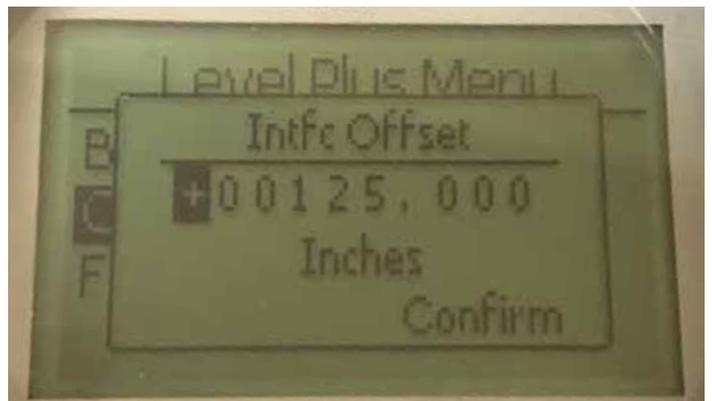
Only used based on Factory Technical Support. If the Interface Level is disabled it will show Not Enabled on the display as shown in section 9.2.1.2.3.2.
