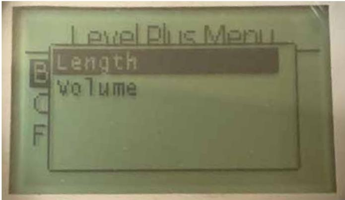
**Length** – Changes display to show the level measurement in the selected units.
