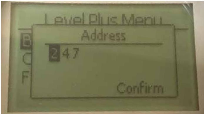
Allows the user to view and change the Modbus address.
