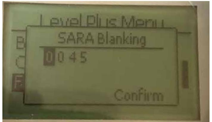
Allows the user to adjust the blanking window for the interrogation pulse. RefineME and SoClean should be at 25 and Tank SLAYER and CHAMBERED at 40. Do not adjust without talking to Temposonics Technical Support.
