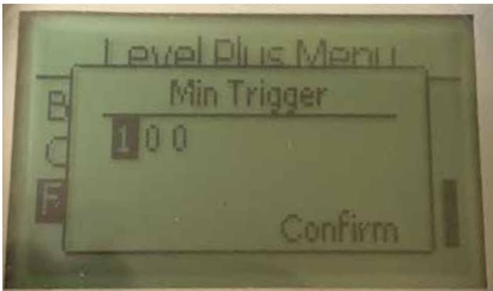
Allows the user to adjust the threshold for which the return signal must meet. The default setting is 150. Do not adjust without talking to Temposonics Technical Support.
