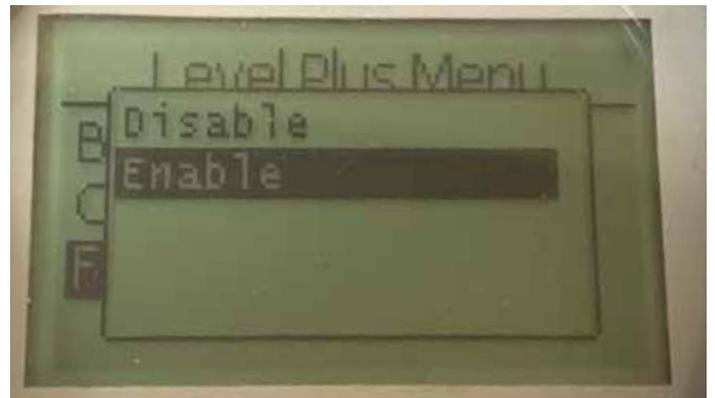
Allows the user to turn the temperature measurement function on or off. Does not enable the function if the unit was not ordered with temperature measurement.
