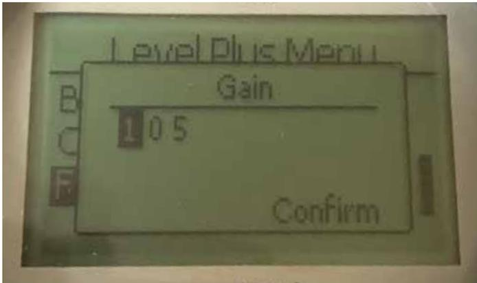
The Gain is the strength of the interrogation pulse. Temposonics uses the same electronics for all lengths and adjusts the signal based on the order length. Do not adjust without talking to Temposonics Technical Support.
