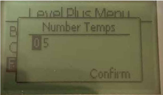
Allows the user to adjust the number of temperature measurement points the level transmitter is looking for. Does not adjust the physical number of temperature sensors that were ordered. Modbus has the option for one, five, twelve, or sixteen temperature sensors.
