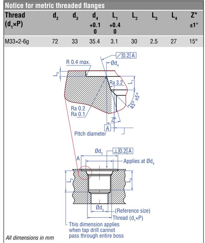
Fig. 4: Cavity dimensions for metric threaded flange M33×2-6h
