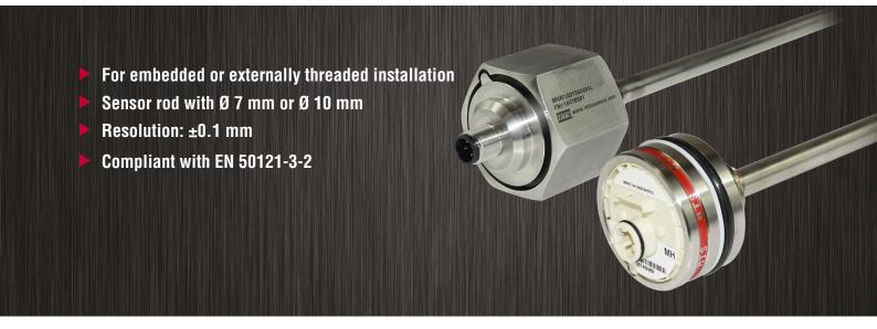
The MHRM sensor extends the rugged design of the Temposonics® MH-Series sensors to railway applications. With two mounting styles, the responsive magnetostrictive linear position sensors can be integrated into most installations. The inherent absolute capabilities ensure that the MHRM sensor is always ready.
