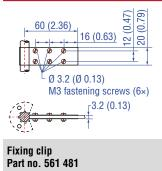
Application: Used to secure sensor rods (Ø 10 mm (Ø 0.39 in.)) when using an U-magnet or block magnet Material: Brass, non-magnetic
