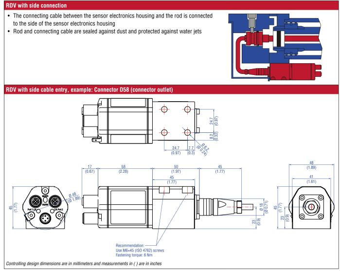
Fig. 3: Temposonics® RDV sensor electronics housing with side cable entry
