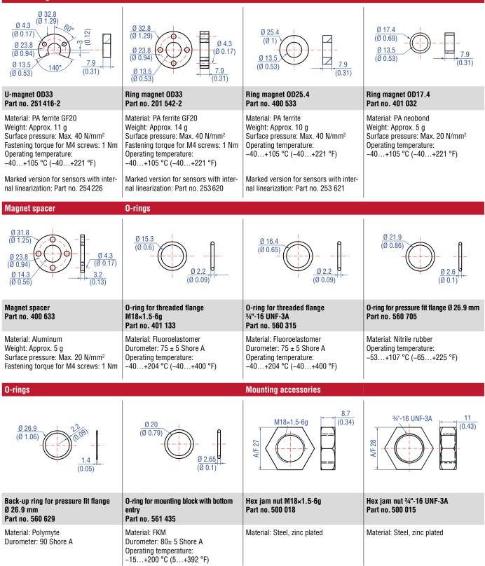
Controlling design dimensions are in millimeters and measurements in ( ) are in inches
