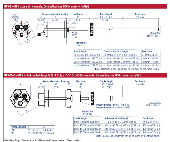
Fig. 2: Temposonics® RFV with ring magnet
