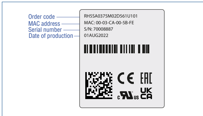
Fig. 1: Example of nameplate of R-Series V RH5 sensor with EtherCAT® output
