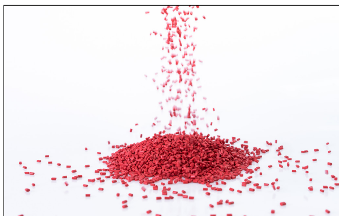
Fig. 2: Plastic granulate for injection molding or extrusion
