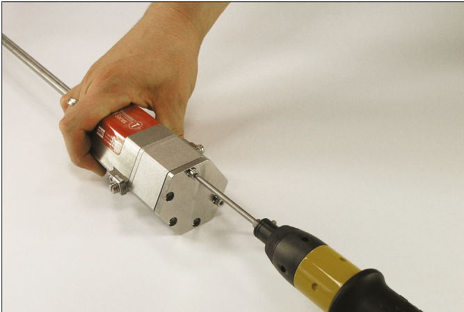
1 Loosen the five M4×10 screws (A/F 3).
