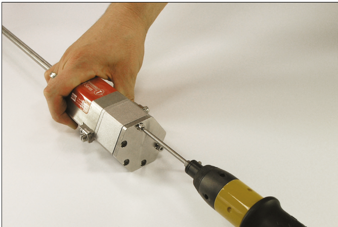
1 Loosen the five M4×10 screws (A/F 3).
