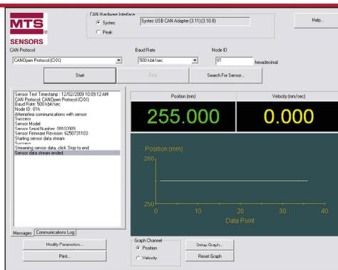
The MH CAN Testkit can be used to perform functional tests and change important settings of TEMPOSONICS MH Sensors with CAN output.
